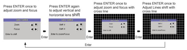
Method 2: Press the MENU button on the remote control and choose Alignment → Lens Control; then use the V▲ ✓ ▶ buttons to adjust the horizontal or vertical position of the lens.
